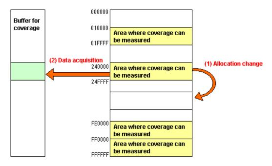
Figure 5.106 Schematic of data coverage memory allocation change
